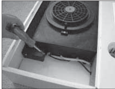
2. Remove two phillips head screws and cover from junction box to gain access to electrical wiring.
